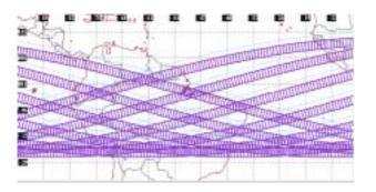
Figure 1 Coverage from an Orbit Inclined at 15°
