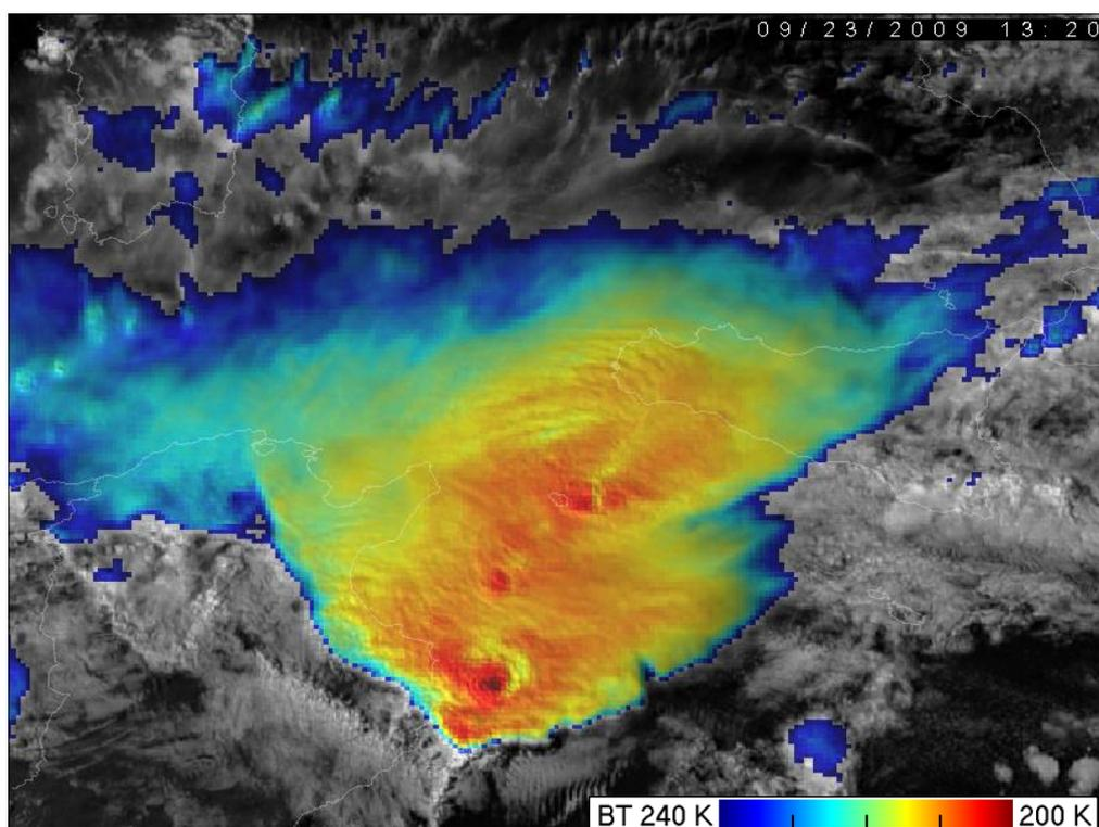
Figure 6. Overshooting tops can be well visualized through a combination of the 1 km HRV channel (providing small scale texture information) and the IR10.8 channel (providing cloud top temperatures). A specific IR10.8 colour enhancement highlights the coldest tops in red. Overshooting tops coincide with severe weather on the ground (hail, wind gusts). An automatic detection scheme is proposed by Bedka et al. (2010).
