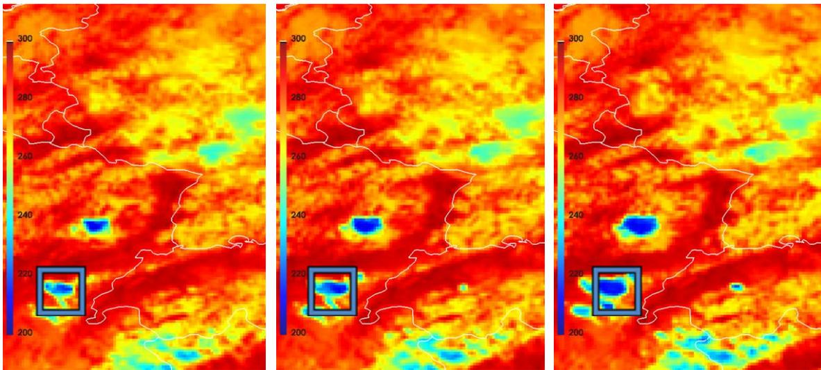
Figure 4. Concept of a the Convective Initiation product: automatic detection of rapidly growing Cu cloud (box), as shown in this sequence of 15 min IR10.8 MSG imagery over Northeastern France (05 June 2007, 1145, 1200, 1215 UTC from left to right).
