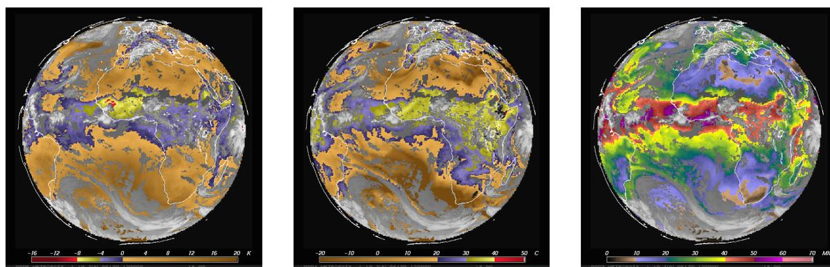
Figure 1. Example of the Lifted Index (left), the K-index (centre) and the total precipitable water (right) as provided by the operational GII product for the entire MSG disk (19 June 2006, 1200 UTC). Detected clouds, where a GII retrieval is not possible, are overlaid in various grey scales to roughly indicate the cloud top temperature.
