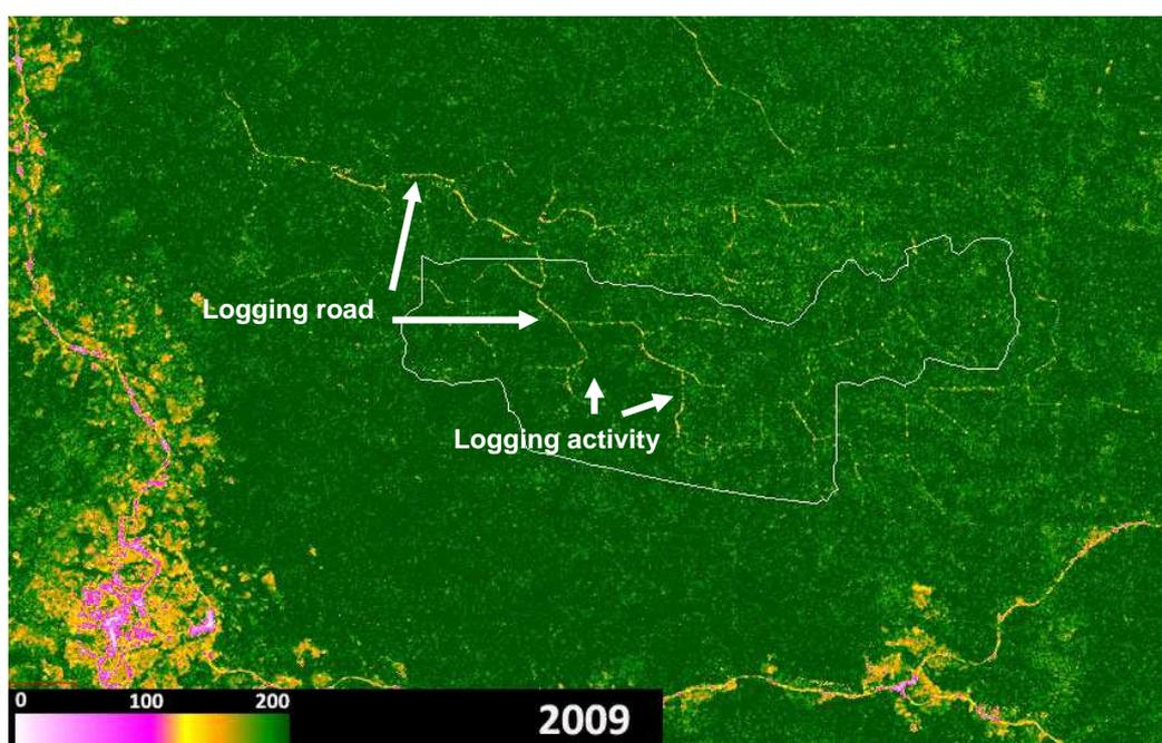
Figure 3. Forest degradation (lighter tones of green) detected by the NDFI index.
