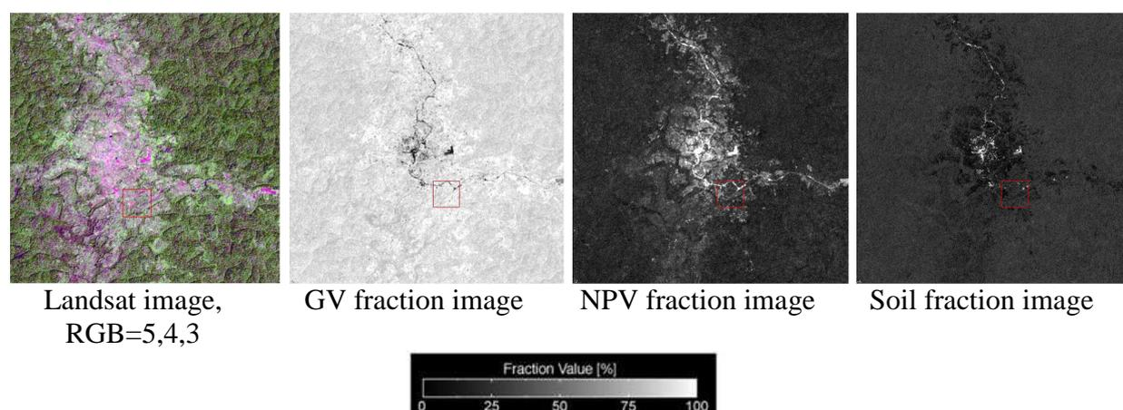
Figure 2. Original image and fraction images resulting from Spectral Mixture Analysis.
