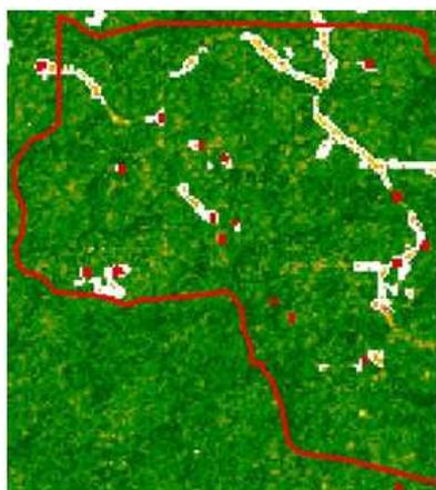
Figure 6c. Log landings (in red) and canopy damage (in white).
