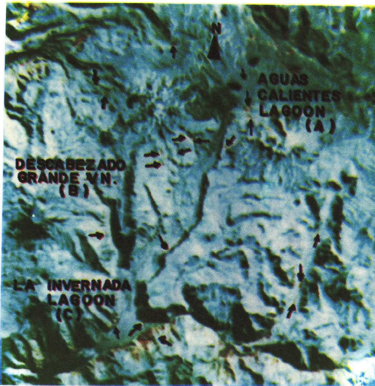
Photo 11. Pilot zone over La Invernada Lagoon sector, to identify geothermal activity through Landsat images. Abnormal snowmelting areas (vegetation spots, water bodies, etc.) near volcanic zones are key elements to be considered.
