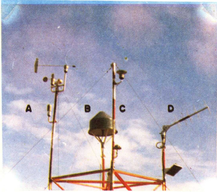
Photo 1. DCP at Marsh Base (A.R.M.C. Presidente Frei), 1978. It is seen: a) mast with sensors b) Landsat antenna c) mast with sensors d) GOES antenna .
