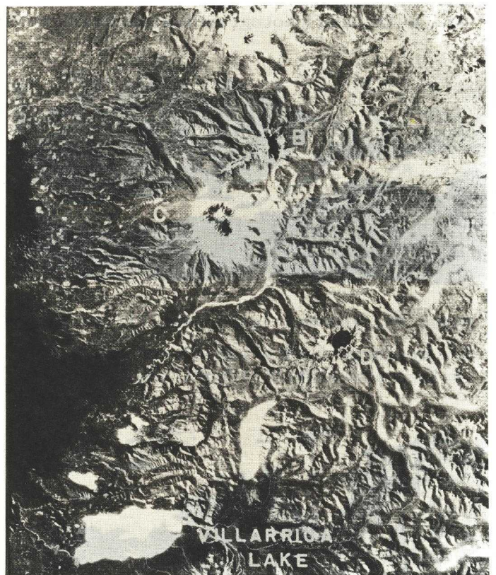
Photo 12b. Band MSS-7 over the same zone of photo 12a, clearly shows the abnormal snowmelting over active volcanoes (indicated through the humid soil, in black tones).
