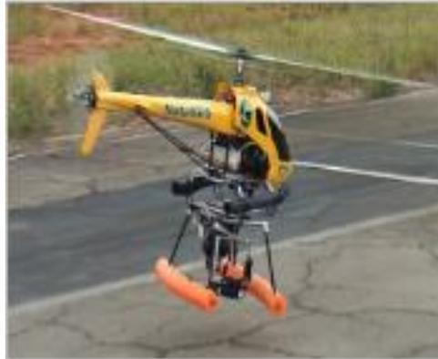
Figure 2: The small helicopter with the pan-tilt image and video acquisition head
