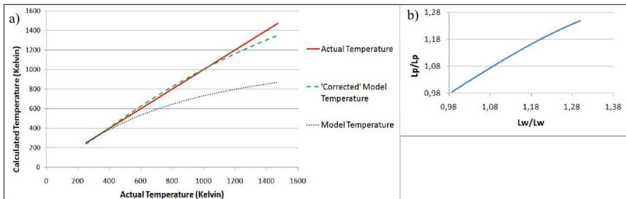
**Figure 1. a)** The relationship between actual temperature, model temperature [i.e. equation [3]] and 'corrected' model temperature, which is based on **b)** the linear relationship between Planck spectral ratios ( $L_p/L_p$ ) and Wien spectral ratios ( $L_w/L_w$ ) for a temperature range of  $-20$  to  $1200^{\circ}\text{C}$  (see text).
