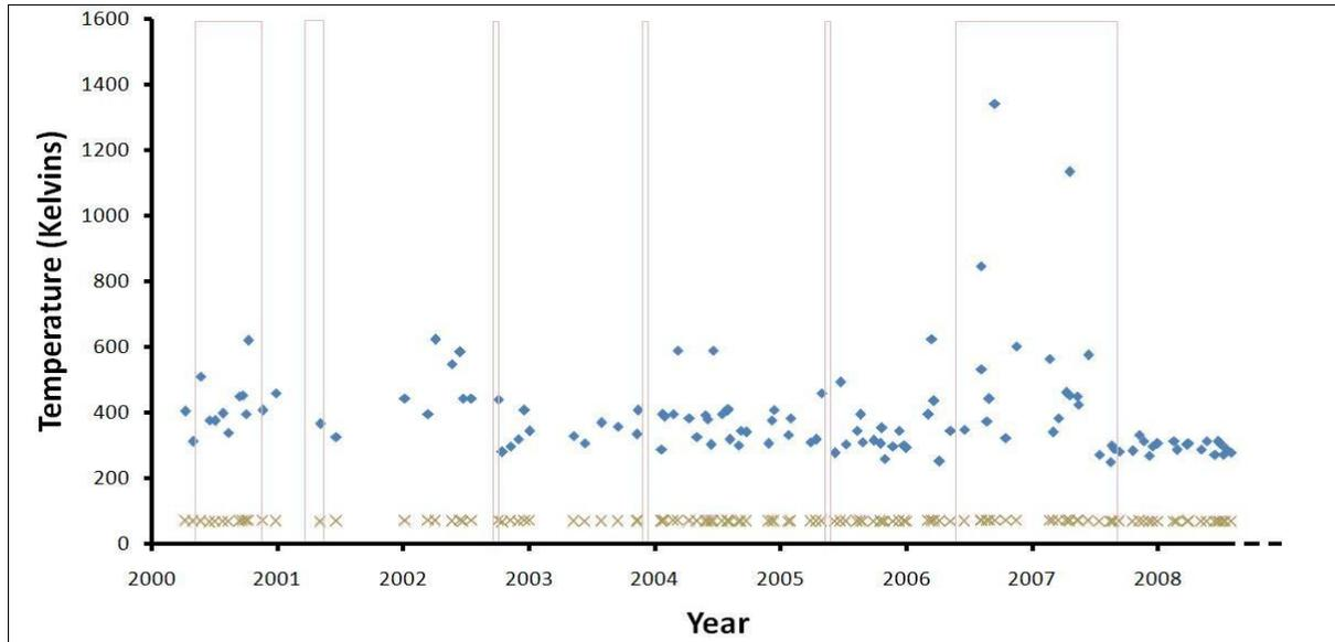
**Figure 2. Temperature Estimates of Lascar volcano using the Grey-body Emissivity Method (GEM) for the 2000-2008 period. The dots are GEM temperatures, the vertical bars indicate the duration and occurrence of the six reported eruptions (Smithsonian Institute). For comparison the brightness temperatures of ASTER bands 13 and 14 are shown respectively as red and green cross-marks.**
