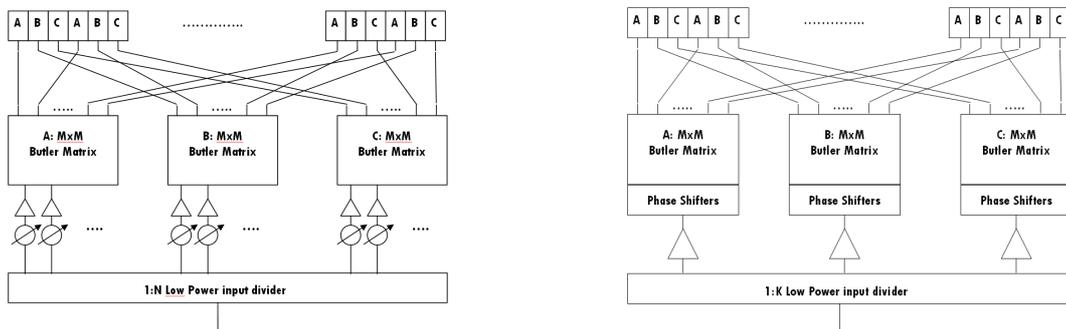
Figure 7 – BFN architecture for maximally low peak power amplifier (left) and for medium/high power amplifier (right).
