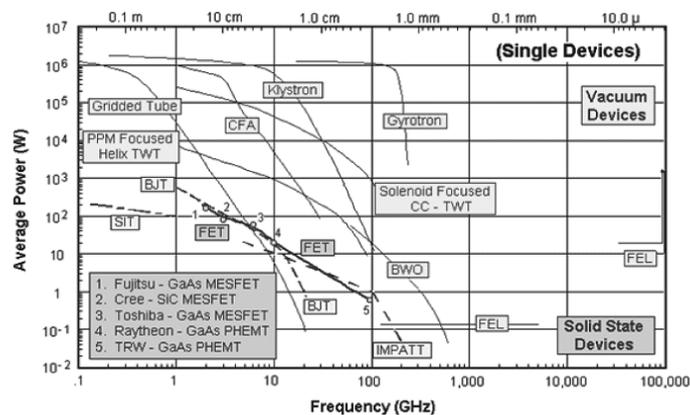
Figure 3 – Available average power versus frequency for single device and for on-ground applications [1]
