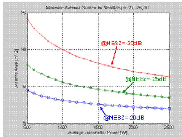
Figure 2 – Antenna area versus average transmitted power for a given NES0
