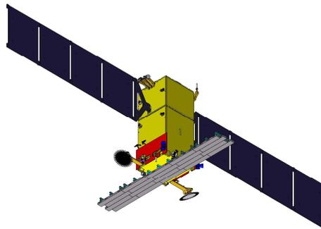
Figure 5 – Example of “Active” antenna SAR satellite configuration for inclined orbit
