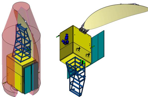
Figure 8 – Stowed and deployed “reflector” antenna configuration
