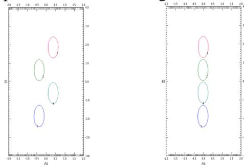
Figure 6 – Typical achievable beam footprint by stacked feed cluster configuration (left) and by long linear array of shared apertures (right)
