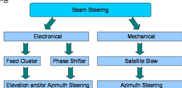
Figure 1 – Beam steering possibilities
