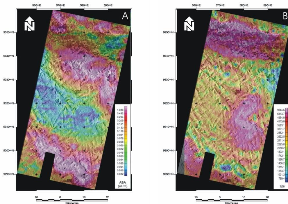
**Figure 1** – Image fusion of simulated MAPSAR and aerogeophysical images: (A) MAPSAR fused with magnetometric image (amplitude of analytical signal); (B) MAPSAR fused with gamma-spectrometric image (total count channel).
