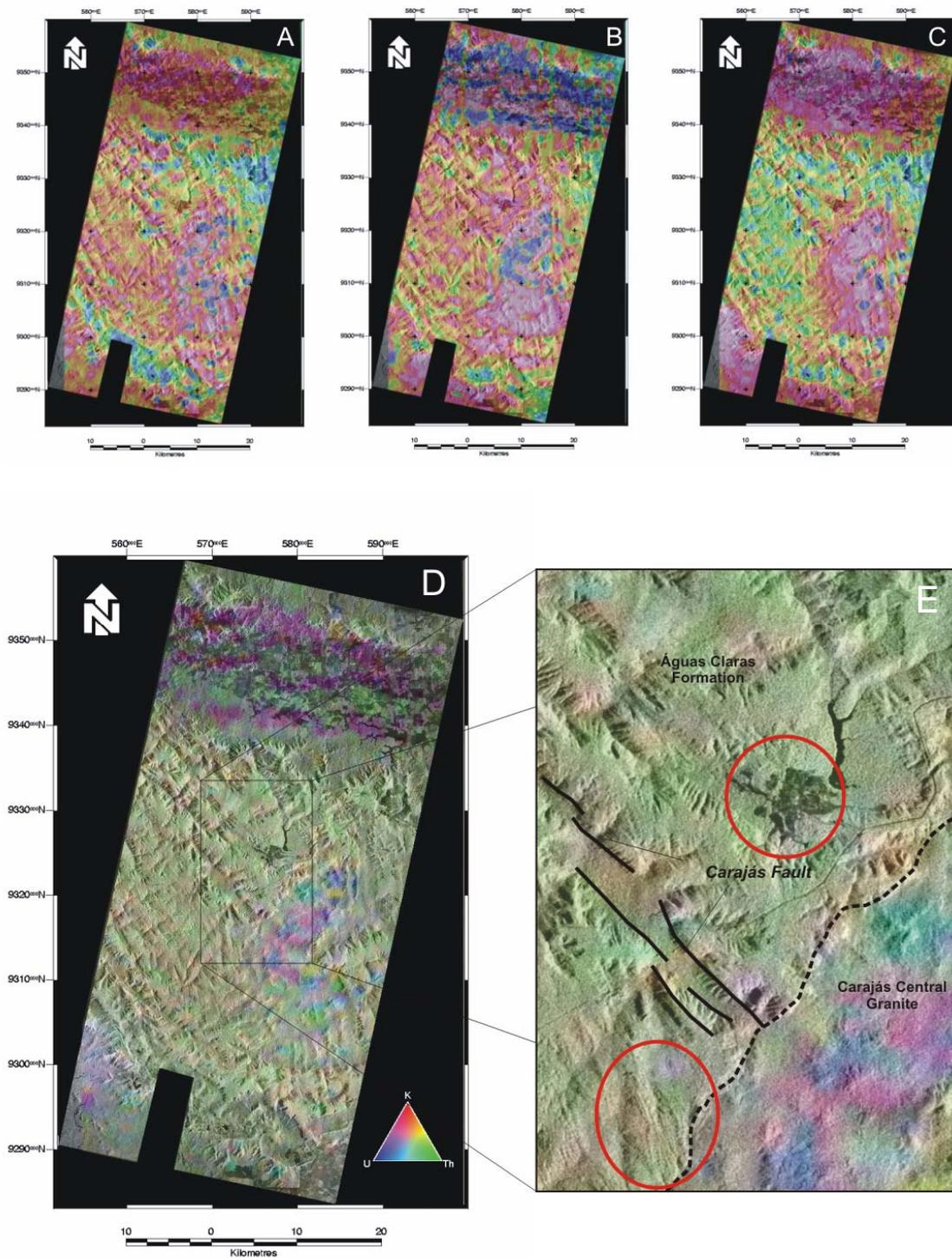
**Figure 2** – Image fusion using simulated MAPSAR and airborne gamma spectrometric images: (A) K channel; (B) Th channel; (C) U channel; (D) color composite of K-Th-U in RGB. (E) Detail of figure 2D for comparison with simulated RADARSAT data (see also Figure 4E).
