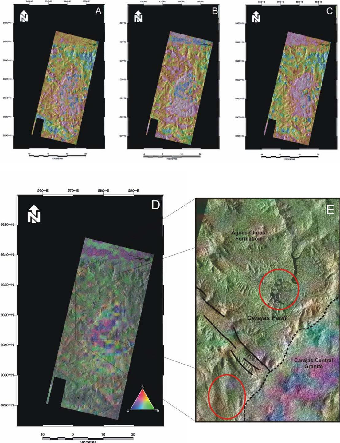
**Figure 3** – Image fusion using RADARSAT (C-Band - Fine mode) and airborne gamma spectrometric images: (A) K channel; (B) Th channel; (C) U channel; (D) color composite of K-Th-U in RGB. (E) Detail of figure 4D for comparison with simulated MAPSAR data (see also Figure 3E).
