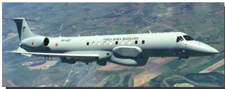
Figure 2- The airborne L-band SAR sensor R99 on board of the EMB-145 aircraft
