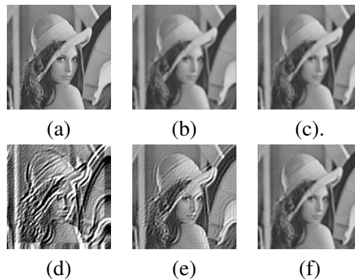
Figure 1: Lena phantom images: (a) Original image. (b) Degraded image. (c) Restored image with \lambda = 0.1 . (d) Restored image with \lambda = 3 . (e) Restored image with \lambda = 1.5 . (f) Restored image with \lambda^* = 0.315026 .
