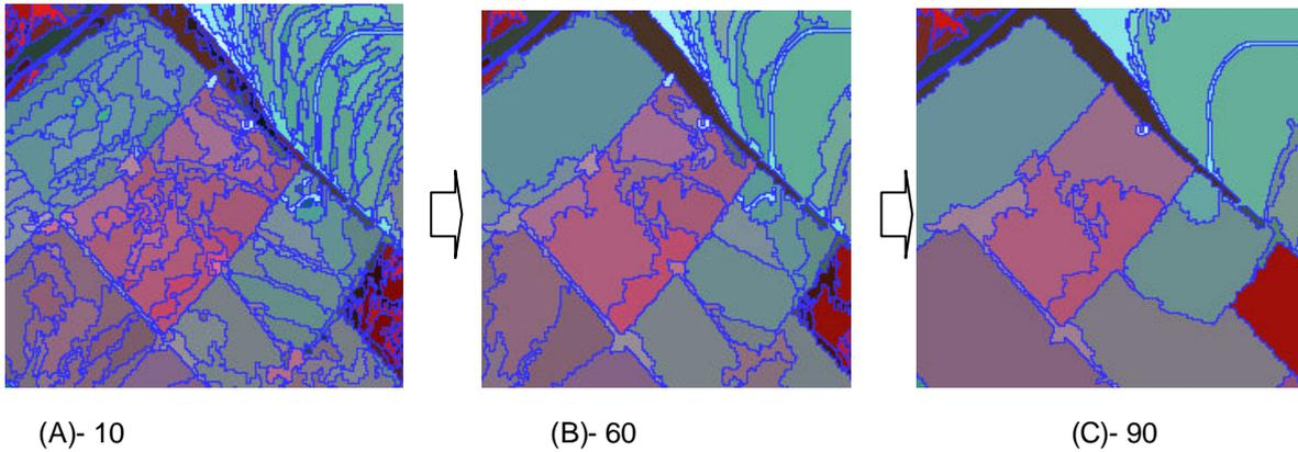
Figure 2- Image segmentation using three different scale parameters
