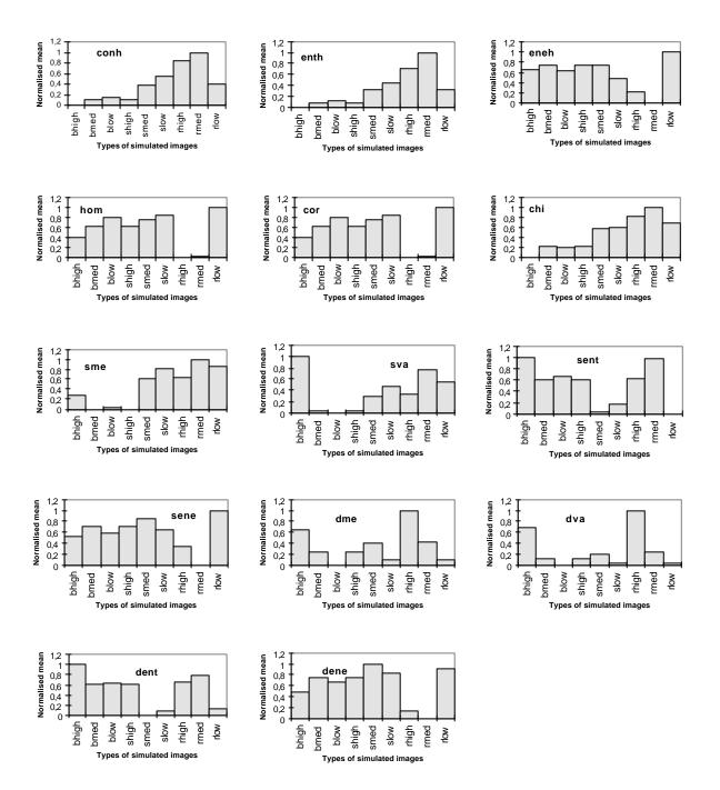
Figure 2. Normalised mean values of GLCM and SADH derived texture measures from simulated images. Codes for the simulated images are: b for big clumps, s for small clumps and r for random; high, med and low for high, medium and low contrast.
