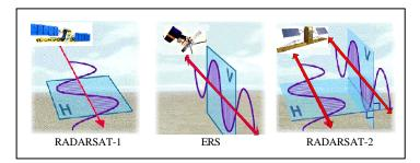
Fig. 1. RADARSAT-1, ERS, and RADARSAT-2 polarization configurations.
