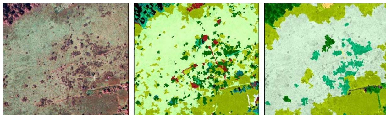
**Figure 1:** Classification of a CIR aerial photograph from 1976. From the original image (*left*), first the level -1 was classified (*middle*) showing high detailed (single bushes in dark green; paths, peat extraction areas in red). Classified image-objects were then aggregated in the focal mapping level (*right*). Bush encroachment is low and the undisturbed active raised bog (bright green) is still dominant.
