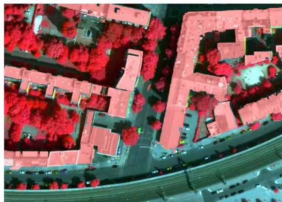
**Figure 2:** Color Infrared (CIR) Aerial Scanner Image (spatial resolution: 0.2m, size: 210m x 150m) (*left*). Extracted Buildings (light red) using advanced Texture and Shape Information in an object oriented software environment (*right*).
