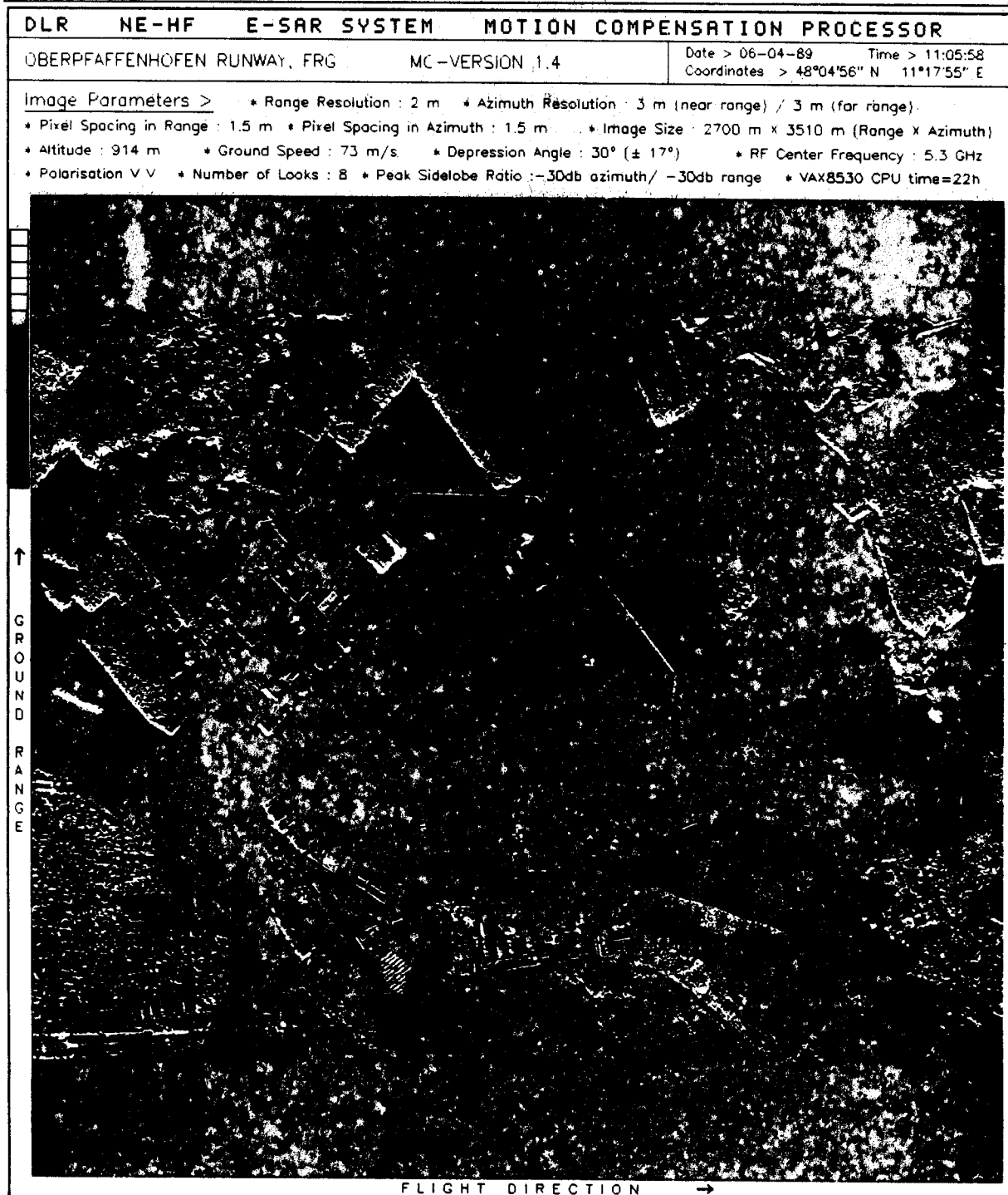
DLR Oberpfaffenhofen Research Centre and Oberpfaffenhofen airfield. E-SAR overflight on April 6, 1989, in C-Band, vertical polarization. Data processed by DLR.
