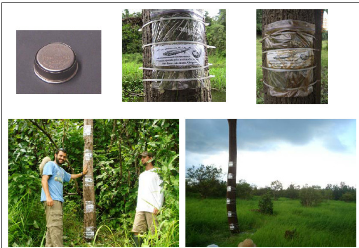
Figure 2: Upper: Thermochron iButton; iButton mount at installation; iButton mount at retrieval. Lower: Examples of iButton stations
