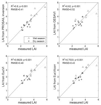
Figure 2. Comparison of measured and estimated LAI from PROSAIL inversion (top left), from GESAVI (top right), from EucVI (lower left) and EucVI<sub>corr</sub> (lower right). Top figures are taken from le Maire et al. (in press). Measured LAI was obtained from destructive sampling.
