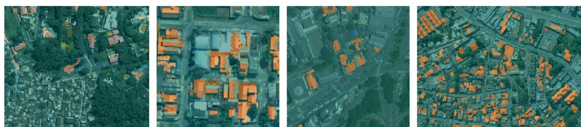
Figure 4: Roof detection in test images (showing full images).
