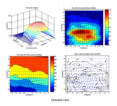
Figure 3: Overland flow characteristics with linear increase, decrease and random variation in Ksat
